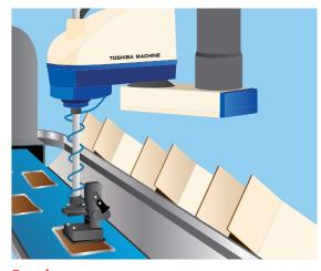
Used for food boxing lines to automatically box ready-packed food being transported on the belt conveyor into boxes.
