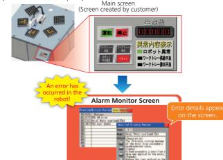
Connection Device Samples is a collaborative system between Toshiba Machine Co., Ltd. and Digital Electronics Corporation. It enables users to check the status of the robot on the touch panel display device.
