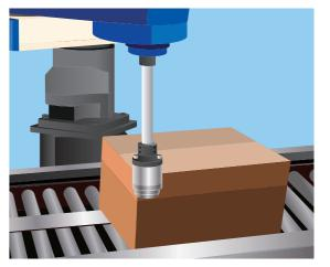
Used as a cutting device. Cardboard boxes being transported by the conveyor are cut by the cutter attached to the SCARA robot.
